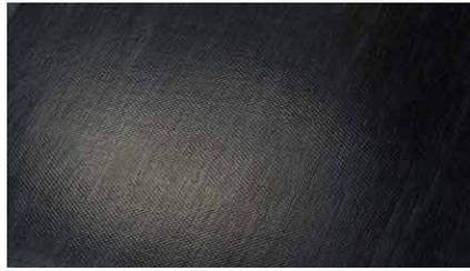
30% lighter than aluminum and has similar strength as steel. Progano semi-finished sheet can be formed in many shapes such as scaffolding boards, concrete casting boards, drainage covers, and other construction applications. Functional elements such as threaded connections and
